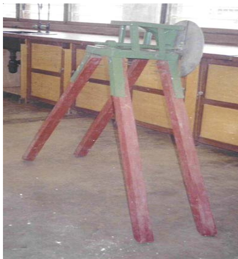
Figure 2: Manually operated slicing machine with wooden legs.
