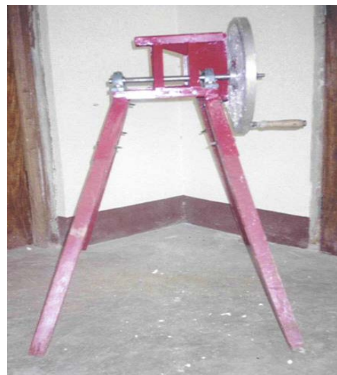
Figure 7: Wooden legged manual chipper with pillow block bearings.
