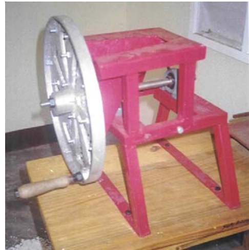
Figure 6: Table mounted manual chipper with pillow block bearings.
