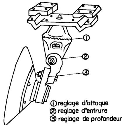
Figure 3. Stanchions with capability of being adjusted for spacing, angle of cutting edge, deviation from vertical and depth.
