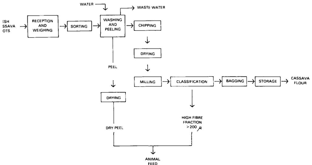
FIGURE 4. FLOW DIAGRAM OF CASSAVA FLOUR PROCESSING PLANT
