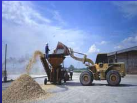
In Thailand cassava roots are chipped and sundried on large concrete drying floors
